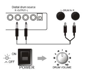
Connect your digital drum set via audio cable to the Drum IN socket of the amplifier while it is switched off.
