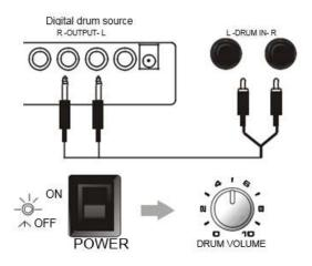
Connect your digital drum set via audio cable to the Drum IN socket of the amplifier while it is switched off.
