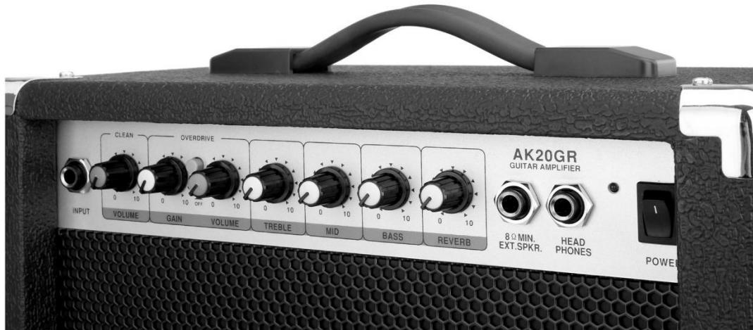
**Volume Clean:** This knob can be used to adjust the volume in the clean channel
