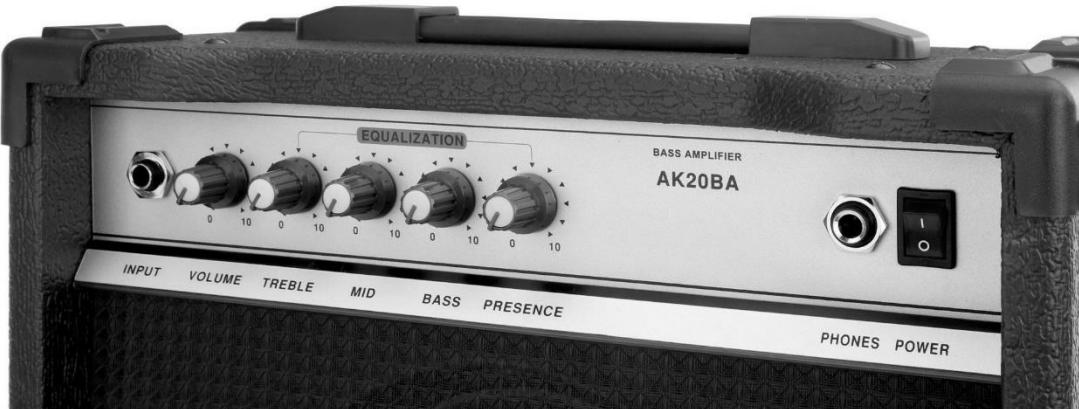
**Volume:** This knob can be used to adjust the volume in the clean channel
