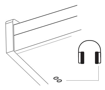
The two 6.3mm headphone jacks on the underside of the console can be used simultaneously. When connecting headphones, the instrument's speakers are deactivated.
