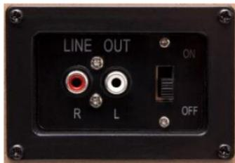
If you operate the jukebox with the integrated speakers, set the switch on the black LINE OUT display on the back of the box to **OFF**. If you want to connect external speakers (LINE OUT) then slide the switch to ON and use the cinch- plugs as indicated.
