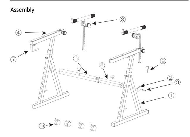
Push the insertion rod **(6)** into the cross bar **(5)** and fix it in the appropriate width with the two screws.
