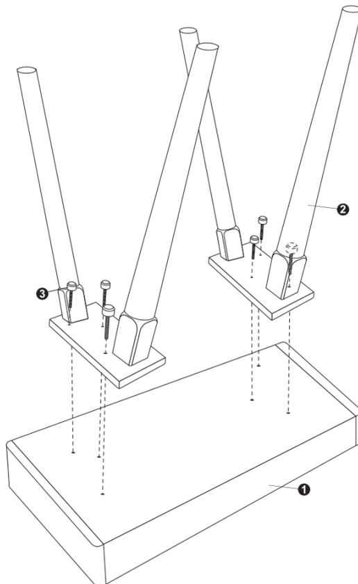
Securely fasten the mounting plates with the assembled support legs (2) to the console using the six plastic head screws (3).
