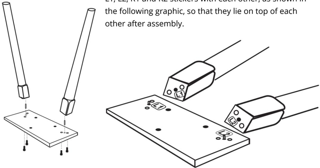
Carefully place the console (1) upside down on a soft surface.
