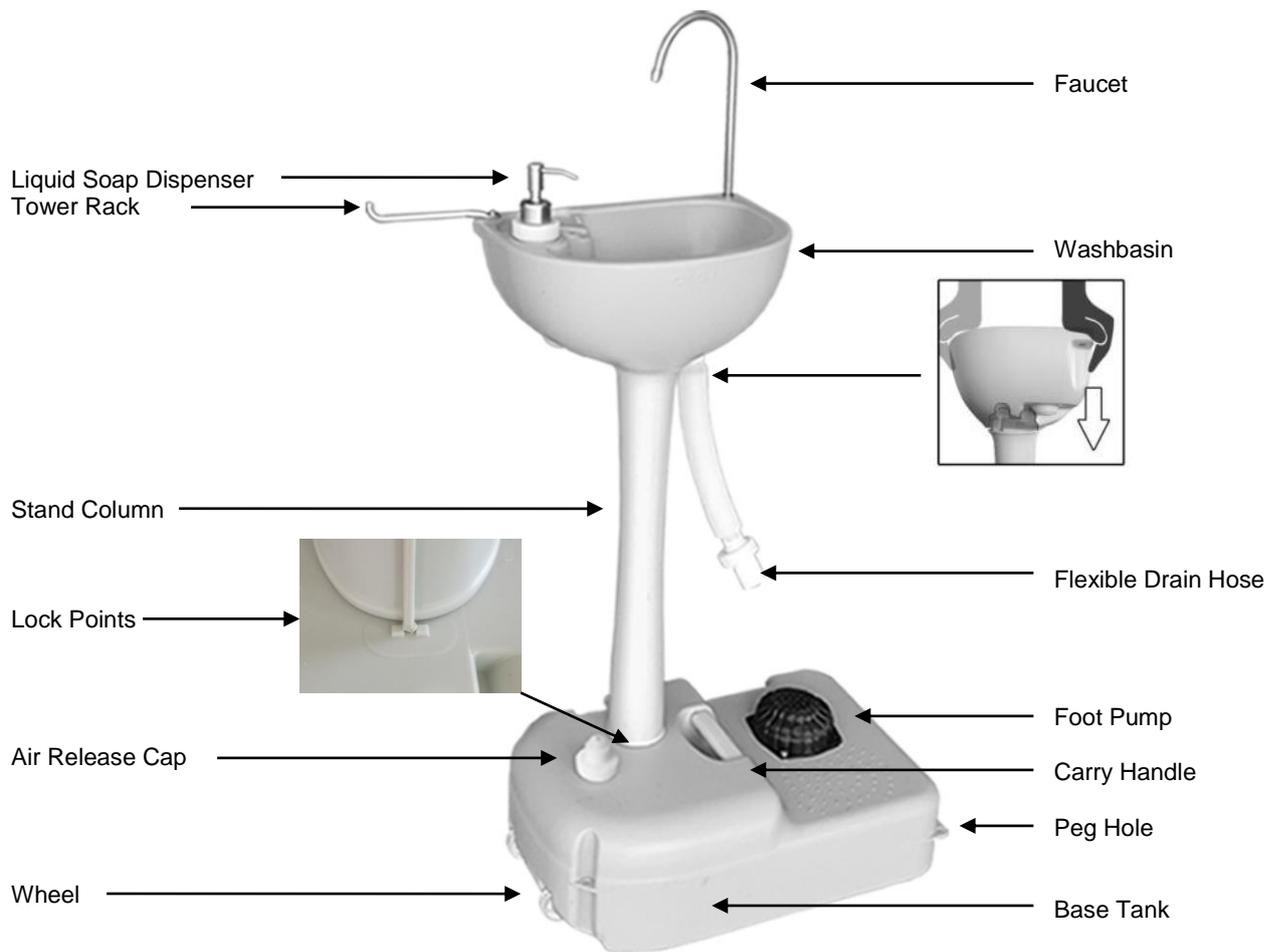
1. Put the washbasin on the ground and press the stand column into the washbasin. Make sure the top of the stand column is fully inserted into the groove of the washbasin and there is no obvious space around.
