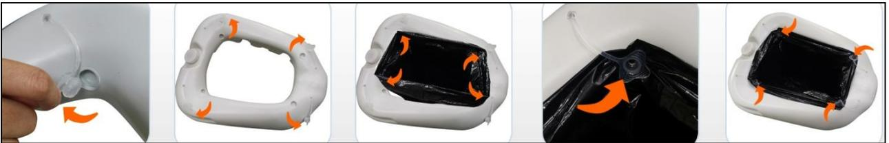
2. Securely attach a plastic waste bag with the clips attached to the toilet seat. Use a bag with a minimum width of 500mm.
