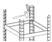
Use a rubber mallet and, if necessary, a slotted screwdriver (both are not included in the scope of delivery) to insert and fix the 20 **cross connections (C)** into the **vertical long struts (B).** The distance between the 5 shelves can be chosen flexibly, but for reasons of stability, make sure that the lowest shelf closest to the floor is max. 150 mm above the floor.
