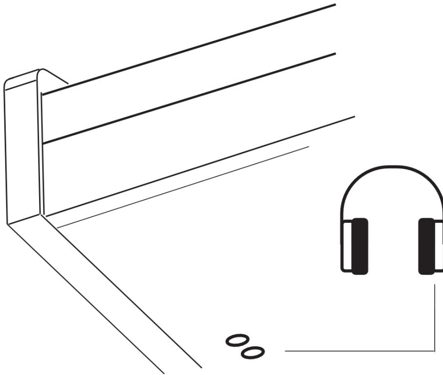
The two 6.3mm headphone jacks on the left rear bottom of the console can be used simultaneously. When connecting headphones, the instrument's speakers are deactivated.
