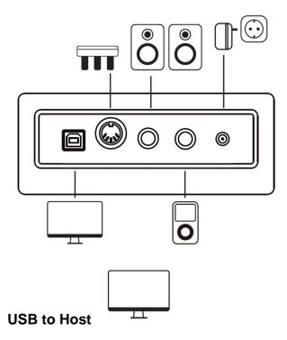
The USB to Host jack allows you to connect your piano to a computer using a USB A->B cable.
