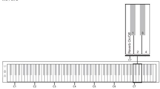
To enhance the room sound of the piano, the instrument has a reverb function. Press the REVERB ON/OFF key while holding the function key to deactivate or reactivate the reverb effect. When the reverb effect is activated, four different effect types are available for selection. Press one of the Reverb 1-4 buttons (1=Room, 2=Hall1, 3=Hall2, 4=Church) while holding the function button to select.
