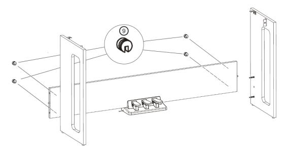
Securely fasten the console ① to the base using the two short M6x20 screws ①.
