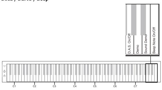
The D.A.S. function (Dynamically adjusted sound) optimally adapts the dynamic range to the selected volume setting in order to provide the maximum dynamic range psychoacoustically at all times. Press the D.A.S. ON/OFF key while holding the function key to deactivate or reactivate this function.
