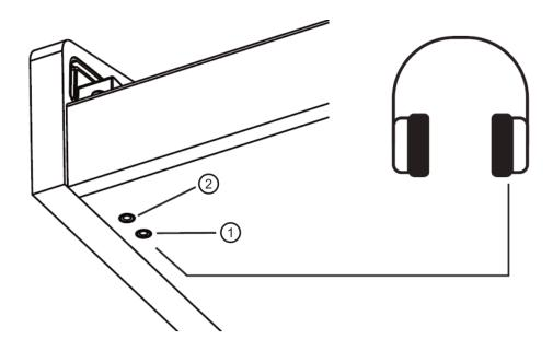
The two headphone jacks on the bottom left of the console can be used simultaneously. When connecting headphones to headphone jack 1, the instrument's speakers are deactivated. When connecting to the headphone jack 2, the sound of the instrument is given out via the headphones and additionally still via the loudspeakers.
