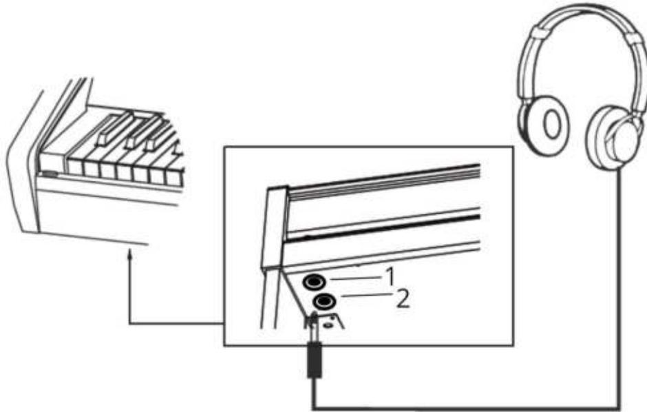
The two headphone jacks on the left underside of the console can be used simultaneously. When connecting headphones to the headphone jack 1, the sound of the instrument is reproduced via the headphones and additionally still via the loudspeakers. When connecting to the headphone jack 2, the instrument's loudspeakers are deactivated.
