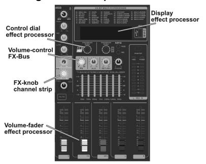
The mixer has an integrated 24-bit multi-effect processor. Turn the knob to preselect the desired effect. Press the knob to activate the effect. On the display, the flashing effect number indicates that an effect has been preselected, and the lit effect number indicates that the effect is active.
