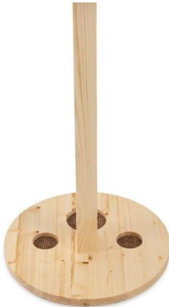
1. Place the rod with the pre-mounted dowels without force on the holes provided. Turn the base plate upwards and fasten it with one of the M8x70mm countersunk screws supplied.
