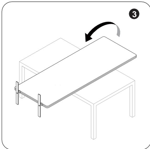
Very carefully rotate the divider panel off of the flat surface and into a standing position. For the best results, make sure the feet are standing on flat and even grounds. Please make sure that feet and panel are connected properly before using the Product.
