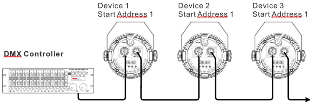
The connecting chain should not exceed a length of 300m or a number of 32 units. Use a terminating resistor at the end of the chain.
