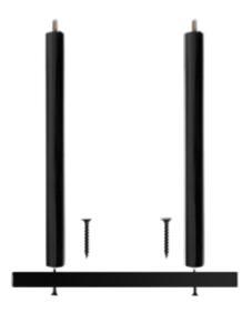
Fasten component (B.) with the supplied wood screws component (G.) IMPORTANT! Make sure that the screws are screwed in centrally.
