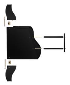
Turn the piano upside down and fix the components (C.) with the screws (L.). Screw components (D.) into the internal threads recessed for this purpose.
