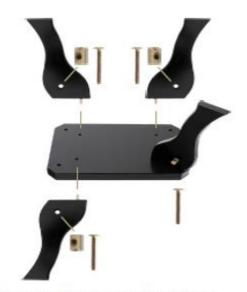
The dowels of the legs (K.) must go into the drilled hole. The legs are fixed by the screws (H.).
