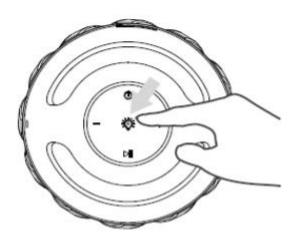
Flame atmosphere lamp ON/OFF Key:Quick press to turn on/off the lamp;Long press invalid.
