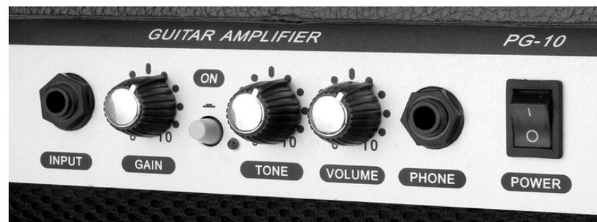
**First steps:** connect your electric guitar with amplifier (**INPUT-jack**) by using the guitar cord. Make sure that **VOLUME** control is set to "0" before you switch **ON** amplifier power.
