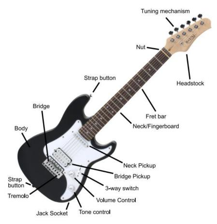
**Jack socket:** Use this socket to connect your electric guitar to an amplifier via a 6.3 mm jack cable.
